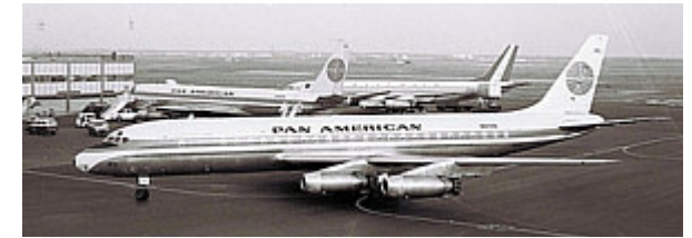
One of sixteen svelte and stylish Pan American Douglas DC-8s. Stretched "Super 70" series, with up to 269 seats, was the largest airliner in service until the lunch of B-747. Because of poor planning and marketing, only 566 were built.
