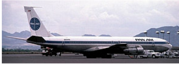
A Pan Am's porky-looking Boeing 707. Boeing people belittled the "ugly" upswept tail and down-sloped nose of the DC-8 but it was capable of accepting a thirty foot stretch while the 707 would drag its tail on rotation if stretched. 1011 built.
