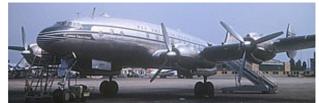
A Pan American Airways Lockheed Constellation. The distinctive triple tail was designed to keep vertical stabilizer height within the height limits of existing hangars. The beautifully curvaceous shape of the fuselage, although hideously expensive to build-- the cross section is not constant-- was designed as a lifting body to reduce drag.
